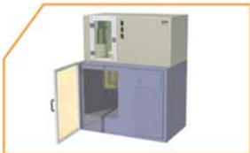
Gelbo Flex with Cooling Chamber
