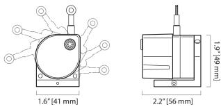
The MT2A is a member of our family of rugged, accurate miniature cable-extension position transducers designed specifically for test applications. One of the major benefits to this sensor its 2-axis 360° rotating mounting bracket to allow for fast and simple installation in any direction.
