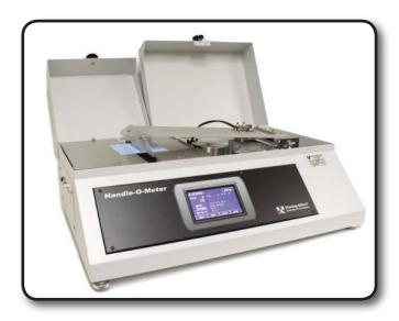
Handle-O-Meter measures the combined effects of flexibility and surface friction of sheeted materials.
