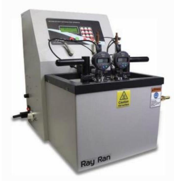
Designed and built to cover multiple international testing standards, the Ray-Ran Advanced HDT/ Vicat Apparatus utilises microprocessor technology to accurately determine the deflection and softening point characteristics of all thermoplastic test specimens.
