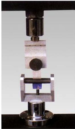
Peeling Test Hard
