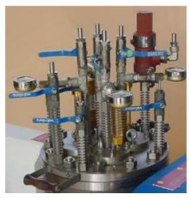
Detail of 4 chamber lid with optional thermometers and pressure gauges.
