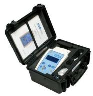
Hypodermic Syringe for plastic packs Septum – Silicon Strip Filters for dry particulate Filters for blocking condensate Sample lines Rugged Carry Case
