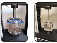
▲ Examples of puncture fixtures used on the Vantage 10 tensile tester. A wide variety of grips and fixtures are available for use with the Thwing-Albert Vantage Series tensile testers.
