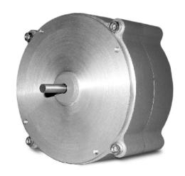
The RT9420 provides rotational position feedback via 4...20 mA current loop signal. This device combines the superb linearity and resolution of a plastichybrid potentiometer and the durability of Celesco's 4...20mA circuit to provide an accurate and reliable electrical signal. Additionally the zero and span settings are adjustable through access holes in the housing.
