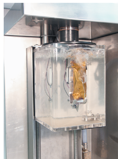
Bubbles emanating from a leak
