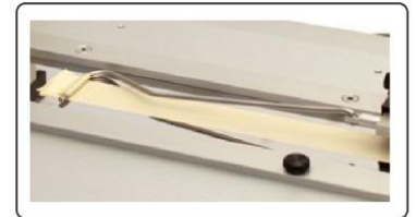
C0055-OP2: 180° Peel Fixture
